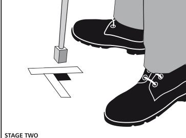
Take the socket block and screw clockwise on to the end of the special insertion tool provided, ensure block is screwed hand tight to the end of the thread. Then using the tool insert the block into the socket.
