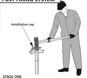
Push Fido socket spike into the ground in a vertical position and insert installation cap into the socket.
